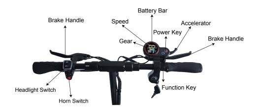
Press the accelerator lightly to speed up the electric scooter.
