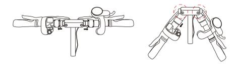
Warm reminder: To make folding more convenient, the ferrule and shaft are not fully tightened, it is normal if there is a gap. Please be assured that this will not affect driving safety.
