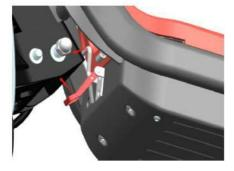
3.When the battery is installed in the frame, first adjust the combination lock to "unlocked state". This step is very important to avoid crushing the internal iron plate.
