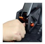
Squeeze the front and rear brakes with both hands, and step on the folding buckle with your feet
