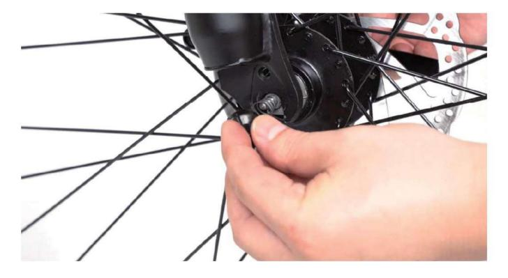
4. Tighten and break the lever upward. Check the position of the wheel.
