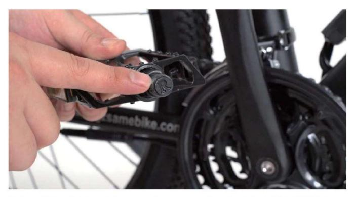
2 . Install the right pedal on the right crankset and rotate it CLOCKWISE to tighten.(Same steps for the left side)
