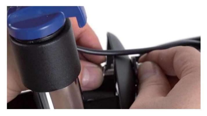
2. Position the headlight and tighten the screws.
