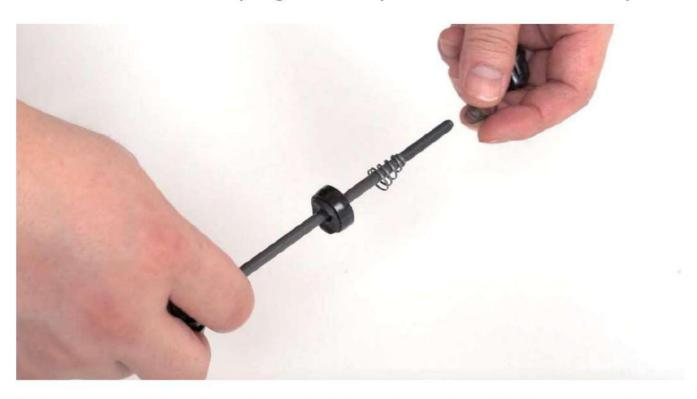
3. Insert the quick release from the left, and then install0 the removed part and tighten the spring and nut on the right in turn, tighten the quick release.
