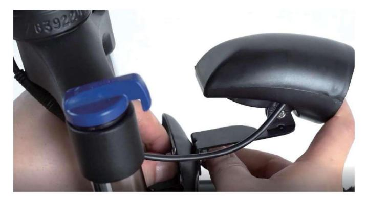
3. Fix the rear fender on the bracket of the seat satys.
