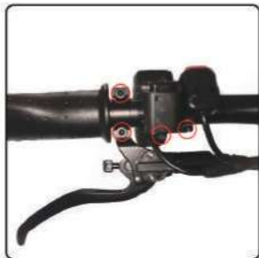
Make sure the brake lever screws and the other two screws are tightened.
