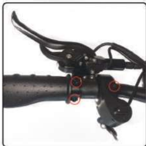
Check whether the brake lever screws and the voltage lockare screws are tightened.
