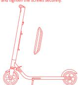
2. Install the support bracket and fasten securely with three screws, as shown.
