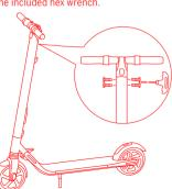
Firmly connect the wires inside the handle and the stem. Slide the handle onto the stem. Be aware of the correct orientation.
