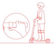
3. Put your other foot on the footrest to keep both feet stable. Press the throttle on right hand to speed up when you are balanced.
