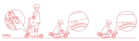
Step on the folding pedal while pushing the handlebar forward slightly. Then fold the handlebar down until it locks into the rear fender.
