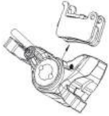
Figure 2-5 Removing/Assembling the Brake Pads and Accessories
