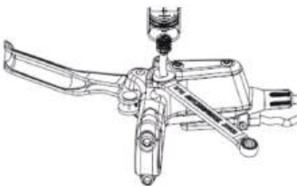
Figure 5-3: 8mm open end spanner to loosen/tighten the main body of the caliper into the nozzle screws.
