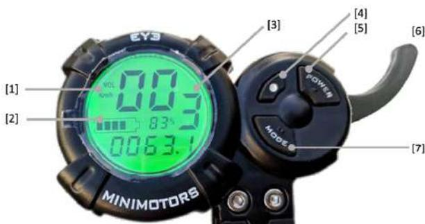
1. *Speedometer.* Shows the speed at which you are travelling.
