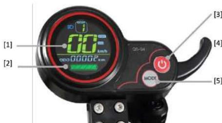
**Gear change.** To change the gear (1=slow, 2=medium, 3=fast), while the scooter is powered ON, press the POWER button to enter gear setting mode. Press MODE to switch between gears. To return to operating mode either press POWER or wait for 2 seconds.
