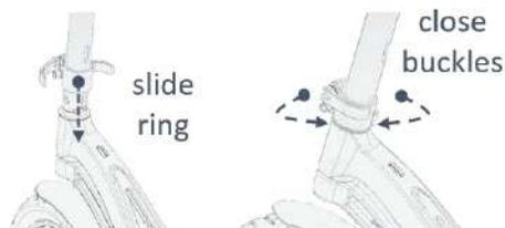
**Before every ride, make sure the buckles are locked tightly around the locking ring.**
