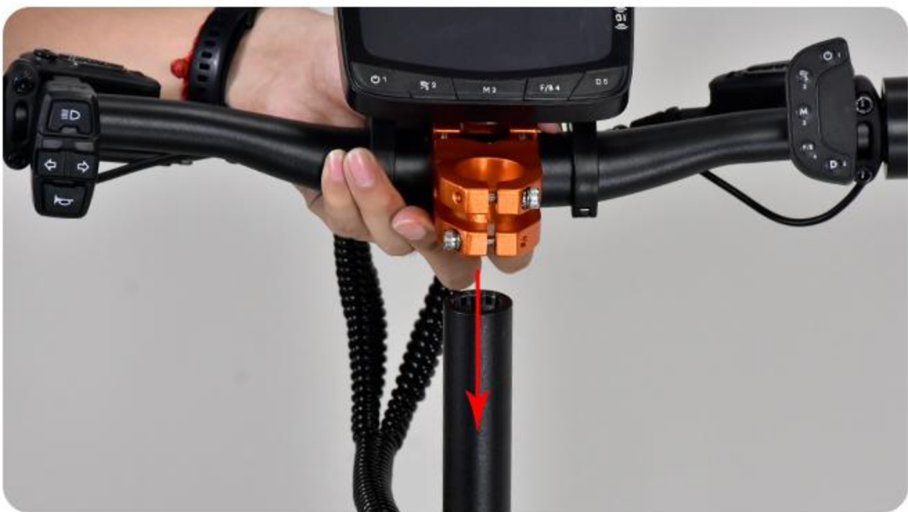
2. Put the handlebar into the handlebar.
