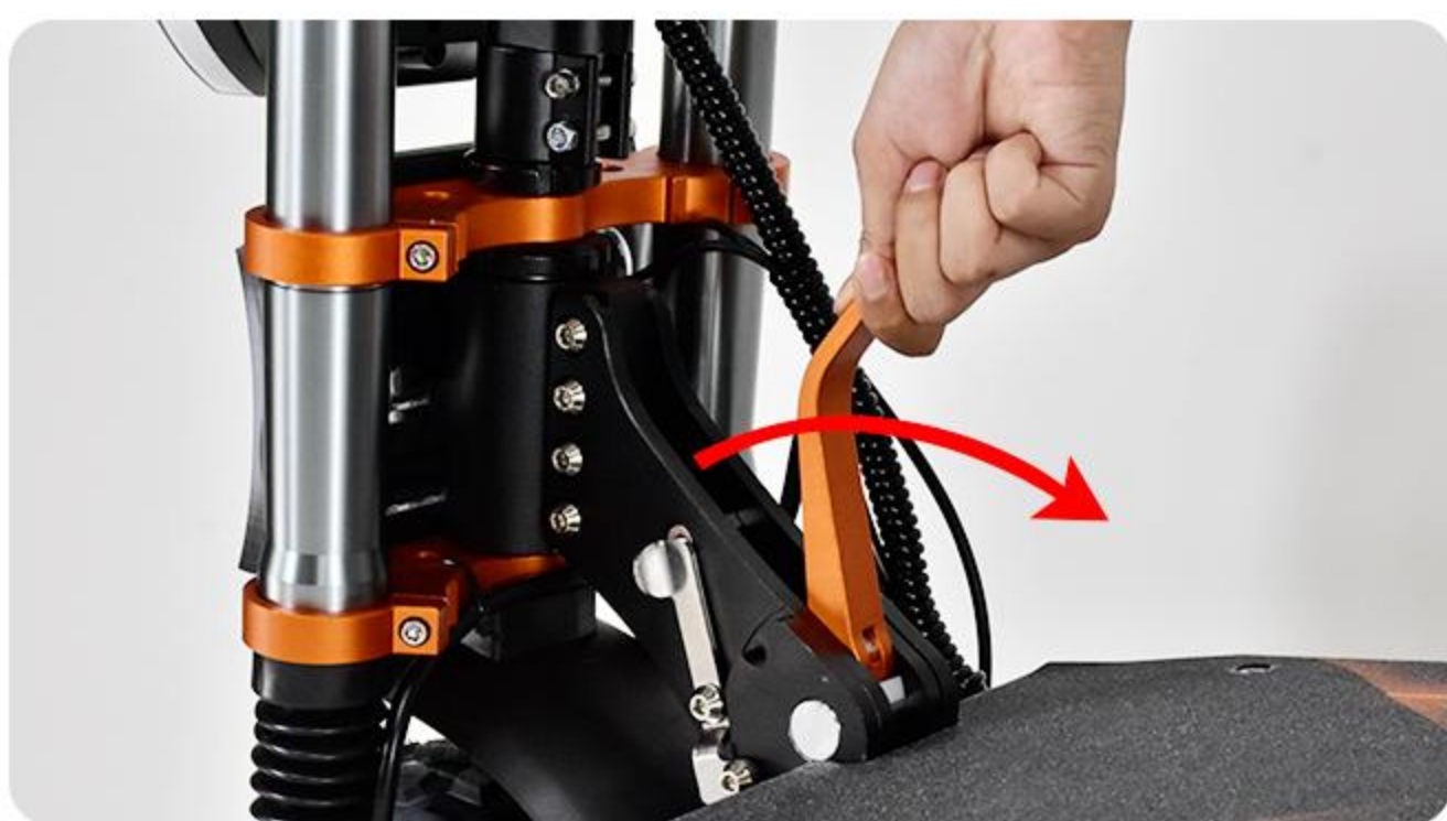
3.Release the stem lock switch
